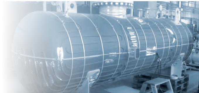
Heating of a tubular screw conveyor with mineral-insulated heating cables. Due to the high temperature resistance of these heating cables temperatures of up to 600 °C can be maintained.
